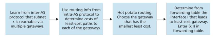
Figure 5.11 Steps in adding outside-AS destination in a router's forwarding table
