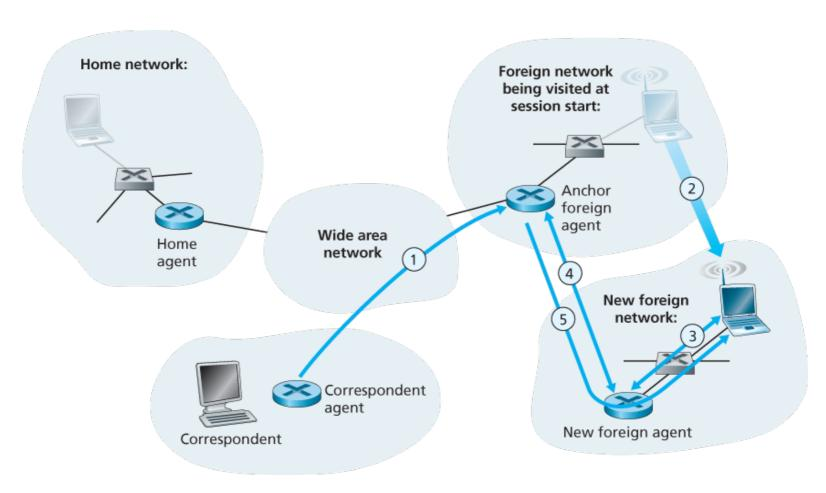
Figure 7.27 Mobile transfer between networks with direct routing
