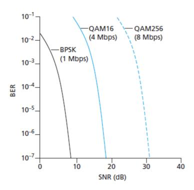
Figure 7.3 Bit error rate, transmission rate, and SNR
