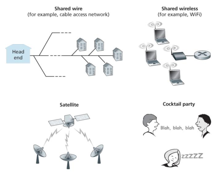
Figure 6.8 Various multiple access channels
