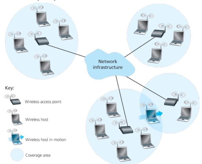
Figure 7.1 Elements of a wireless network
