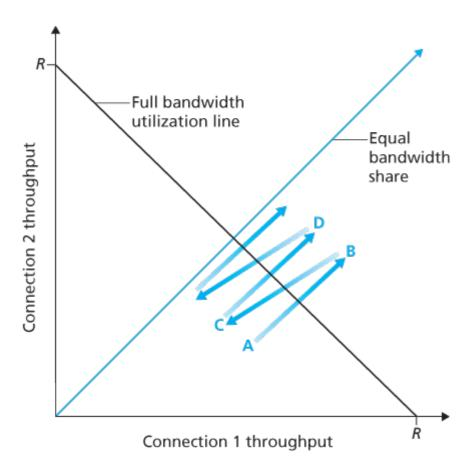
Figure 3.55 Throughput realized by TCP connections 1 and 2
