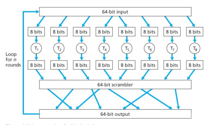
Figure 8.5 An example of a block cipher
