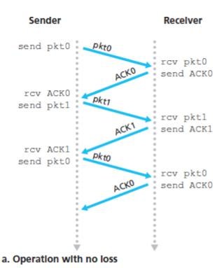
Figure 3.16 Operation of rdt3.0, the alternating-bit protocol
