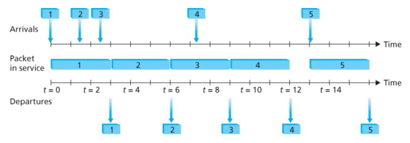
Figure 4.11 The FIFO queue in operation
