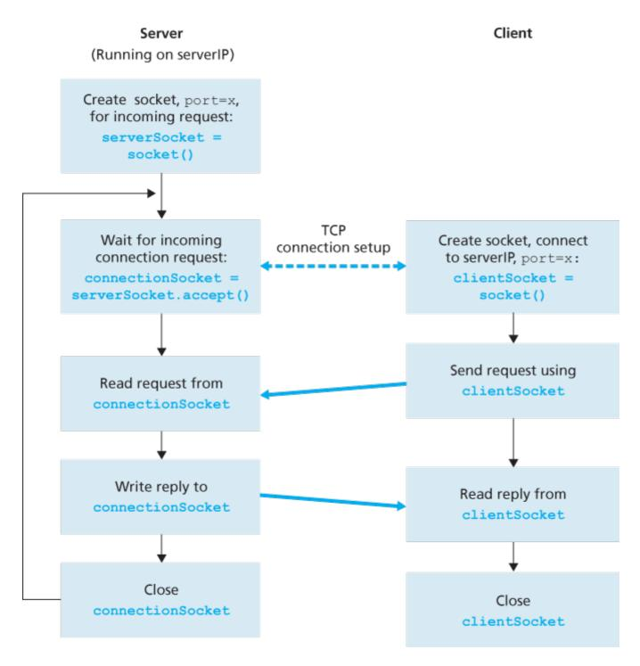
Figure 2.29 The client-server application using TCP
