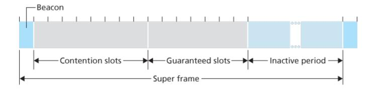
Figure 7.17 Zigbee 802.15.4 super-frame structure
