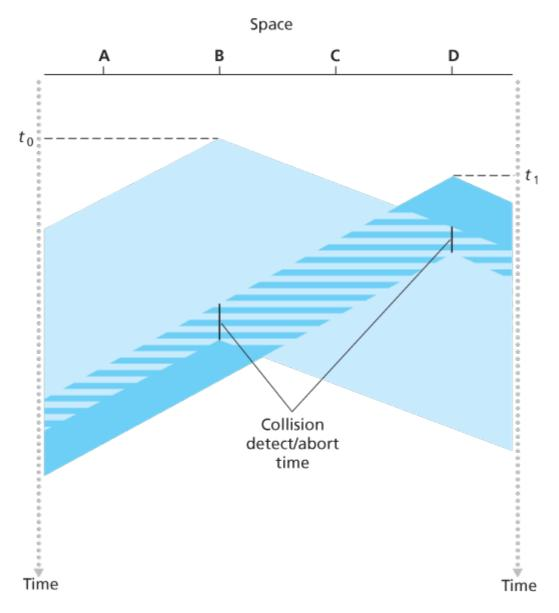
Figure 6.13 CSMA with collision detection
