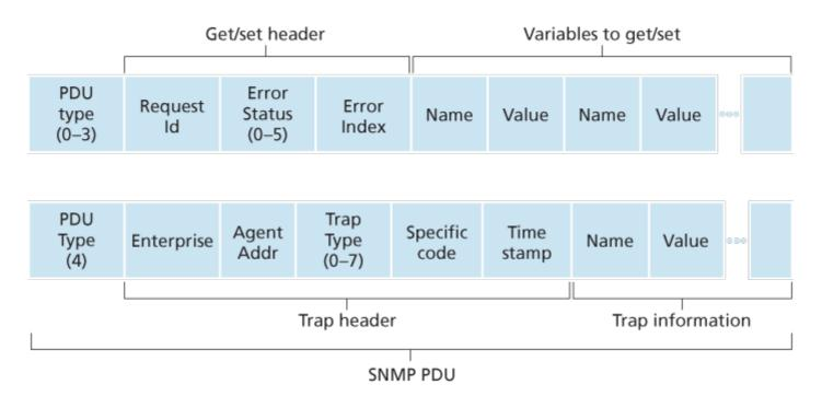
Figure 5.21 SNMP PDU format
