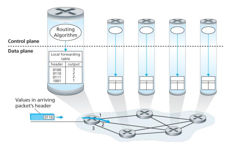
Figure 4.2 Routing algorithms determine values in forward tables
