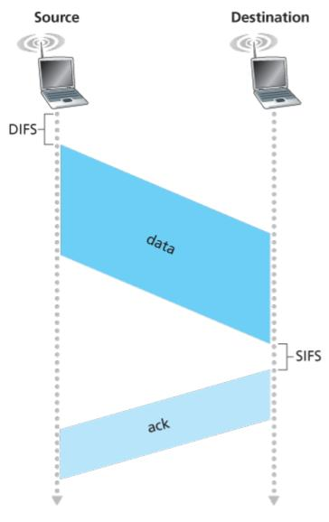
Figure 7.10 802.11 uses link-layer acknowledgments
