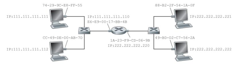
Figure 6.19 Two subnets interconnected by a router
