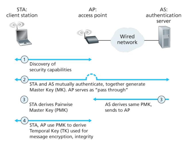
Figure 8.31 802.11i: Four phases of operation
