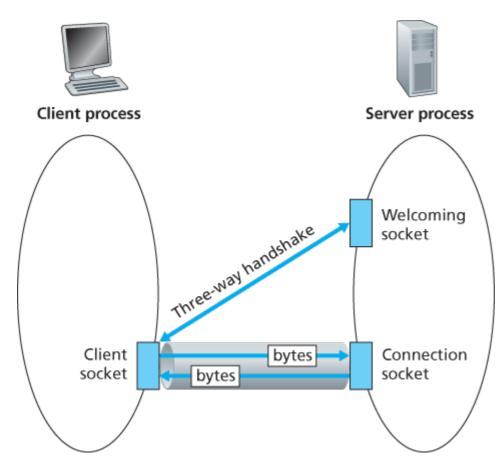
Figure 2.28 The TCPServer process has two sockets
