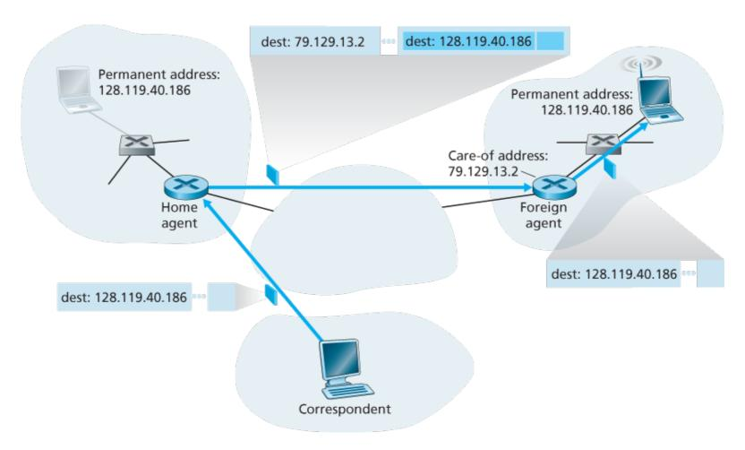
Figure 7.25 Encapsulation and decapsulation
