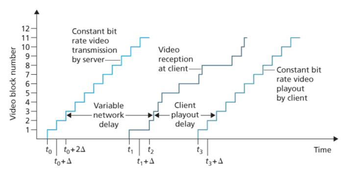
Figure 9.1 Client playout delay in video streaming
