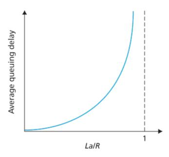
Figure 1.18 Dependence of average queuing delay on traffic intensity
