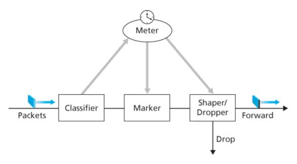
Figure 9.17 A simple Diffserv network example
