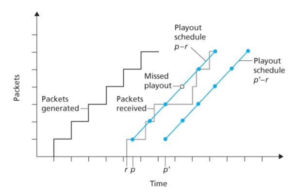
Figure 9.4 Packet loss for different fixed playout delays
