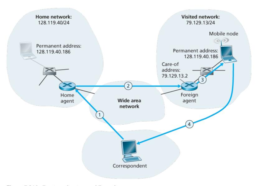
Figure 7.24 Indirect routing to a mobile node
