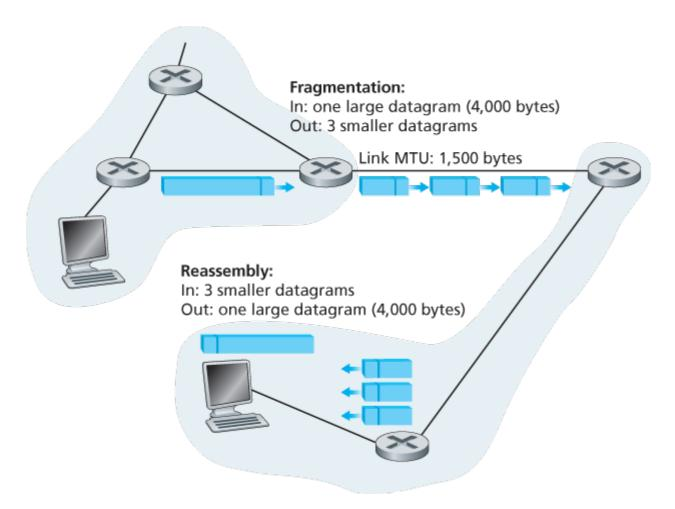
Figure 4.17 IP fragmentation and reassembly
