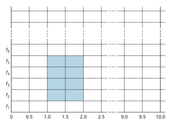
Figure 7.21 Twenty 0.5 ms slots organized into 10 ms frames at each frequency. An eight-slot allocation is shown shaded.
