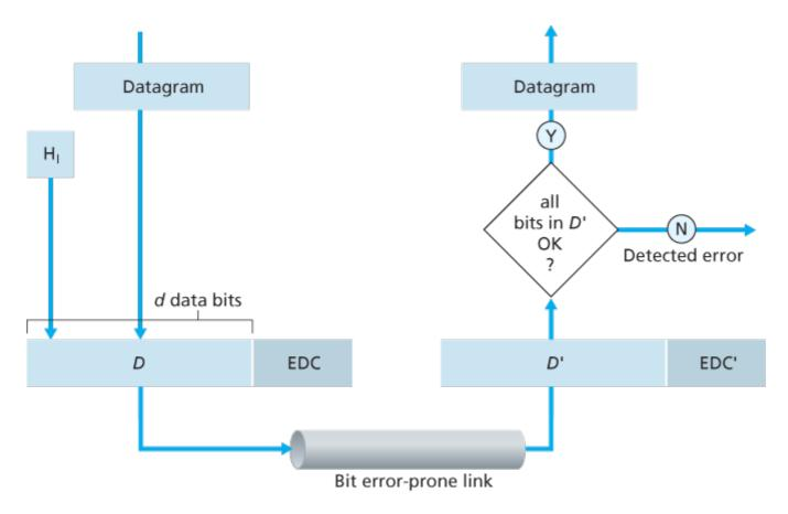
Figure 6.3 Error-detection and -correction scenario
