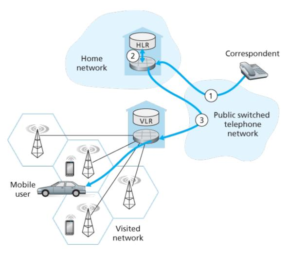
Figure 7.30 Placing a call to a mobile user: Indirect routing
