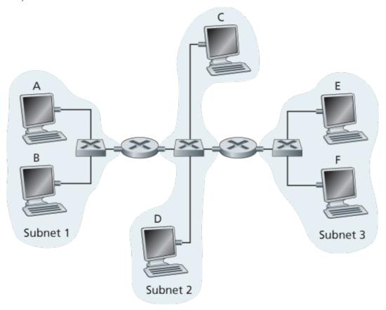
Figure 6.33 Three subnets, interconnected by routers
