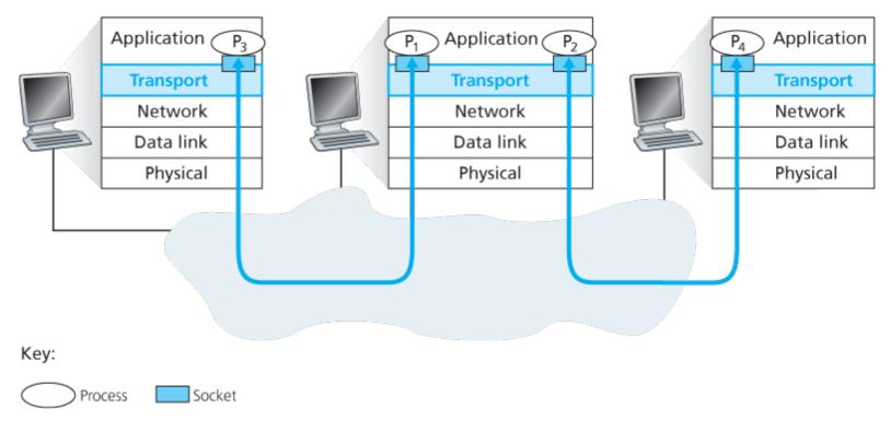
Figure 3.2 Transport-layer multiplexing and demultiplexing
