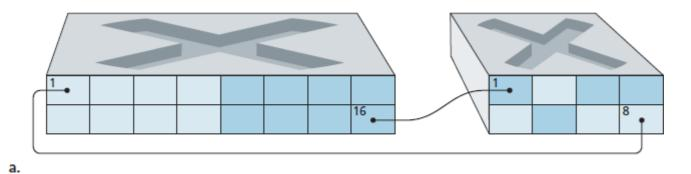
Figure 6.26 Connecting two VLAN switches with two VLANs: (a) two cables (b) trunked
