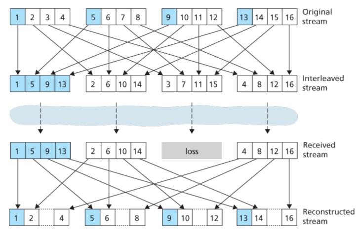
Figure 9.6 Sending interleaved audio
