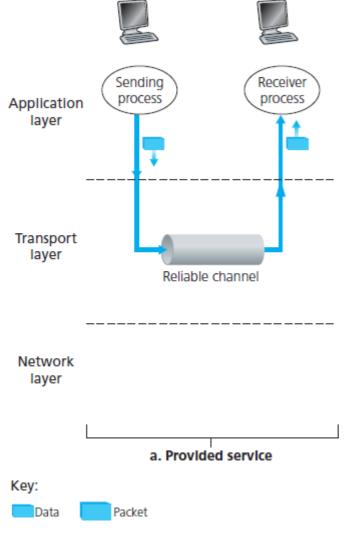
Figure 3.8 Reliable data transfer: Service model and service implementation
