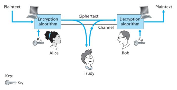
Figure 8.2 Cryptographic components
