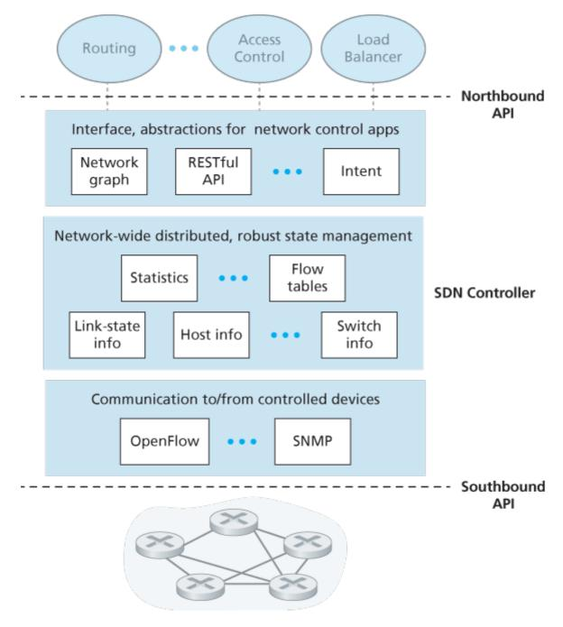
Figure 5.15 Components of an SDN controller
