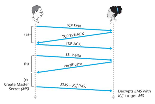
Figure 8.25 The almost-SSL handshake, beginning with a TCP connection
