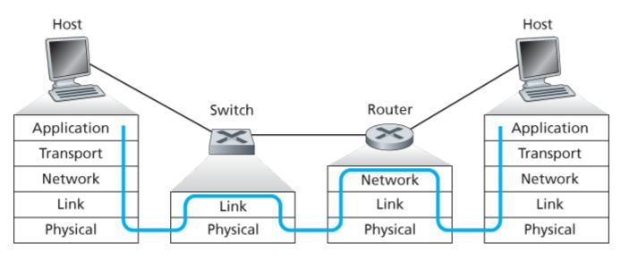
Figure 6.24 Packet processing in switches, routers, and hosts
