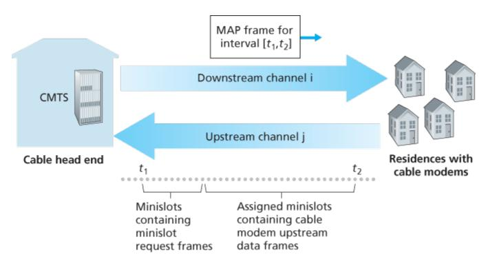
Figure 6.14 Upstream and downstream channels between CMTS and cable modems
