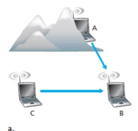
Figure 7.4 Hidden terminal problem caused by obstacle (a) and fading (b)
