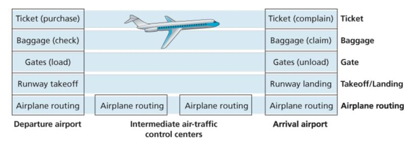
Figure 1.22 Horizontal layering of airline functionality
