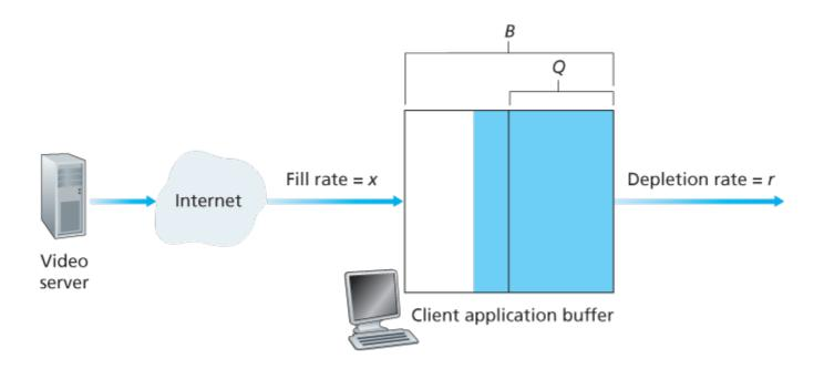
Figure 9.3 Analysis of client-side buffering for video streaming
