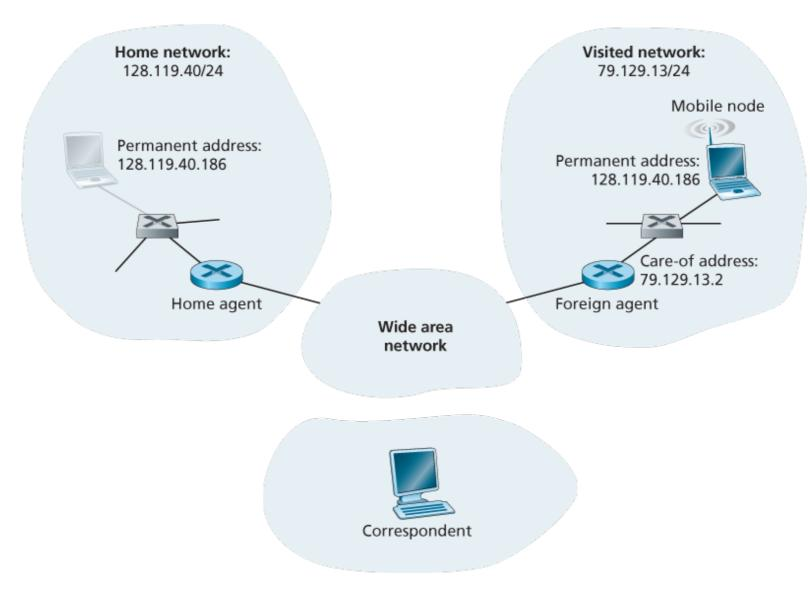
Figure 7.23 Initial elements of a mobile network architecture
