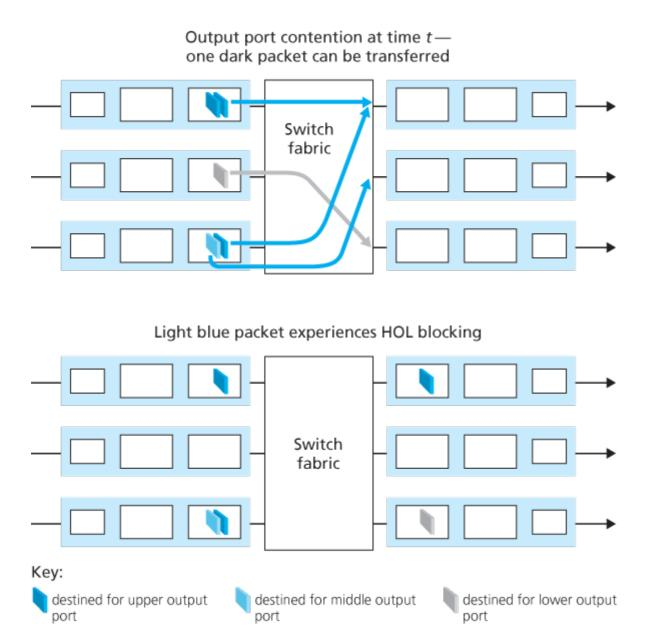
Figure 4.8 HOL blocking at and input-queued switch
